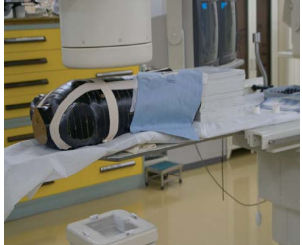
Fig. 1. RANDO phantom with a protective sheet. A protective sheet was placed at the site corresponding to the right lower abdomen on the phantom.
