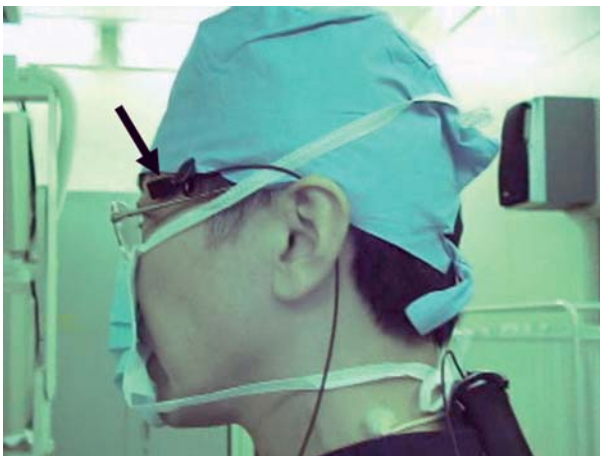
Fig. 2. A probe of the real-time dosimeter (Unfors EDD-30) was attached near the operator's left eye.
