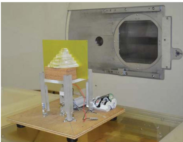
Figure 3. The phantom was divided, and a Gafchromic film was sandwiched in between. The phantom and the stand was positioned on the patient table of the linear accelerator.
