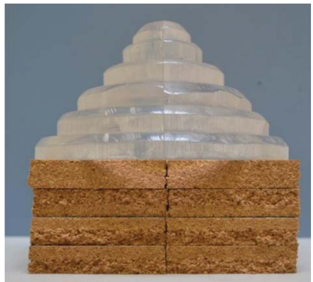
Figure 1. A phantom simulating breast and lung tissues consisted of acrylic boards and cork boards.
